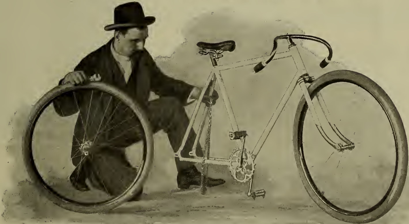
Removing Rear Wheel from Frame Without Disturbing Adjustments or Detaching Chain.
